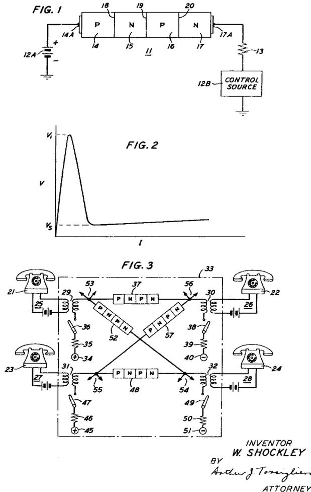
Fig. 15. Shockley's invention of the P-N-P-N four-layer switching diode and its application as a telephone-line cross-point switch (U.S. Patent 2 855 524).
