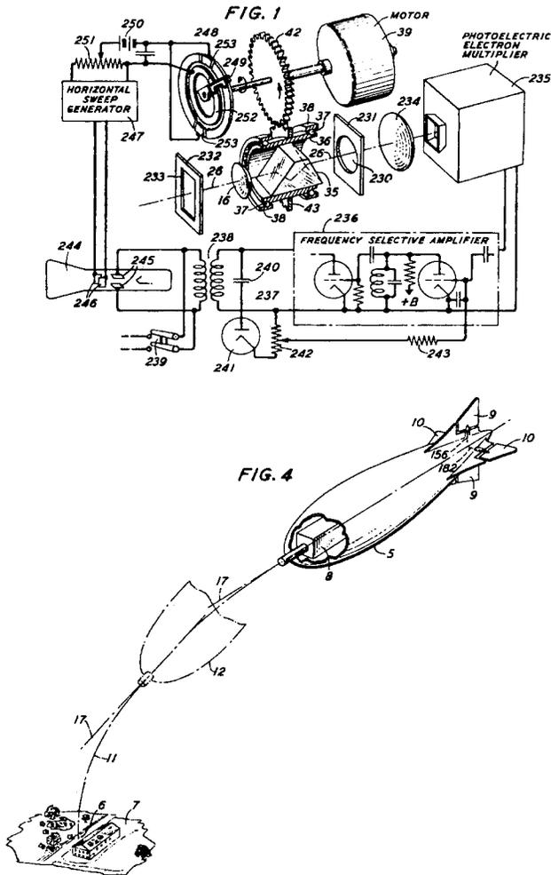
Fig. 7. Shockley's invention of a guided-missile control system that employed the electron multiplier device (U.S. Patent 2 884 540).
