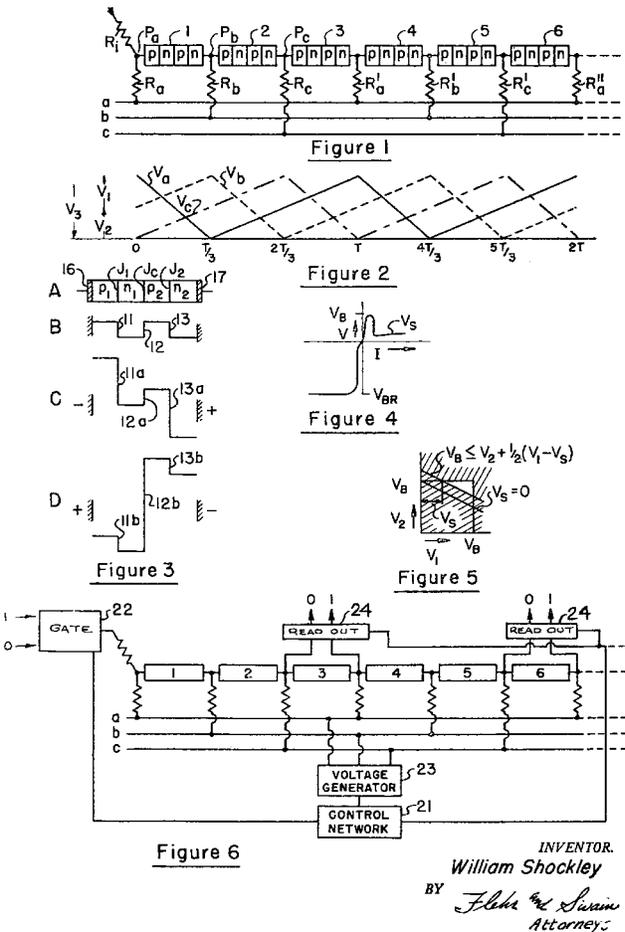
Fig. 21. Shockley’s invention of the semiconductor shift register with four-layer p-n-p-n diodes (U.S. Patent 2912 598).
