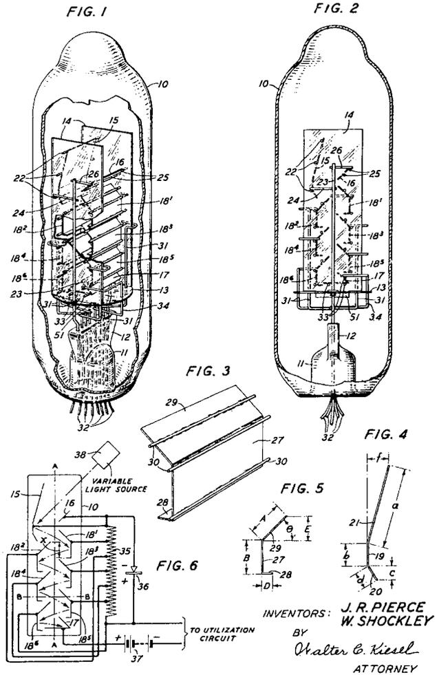
Fig. 6. The electron multiplier tube from the first patent issued jointly to W. Shockley and J. R. Pierce (U.S. Patent 2 245 605).
