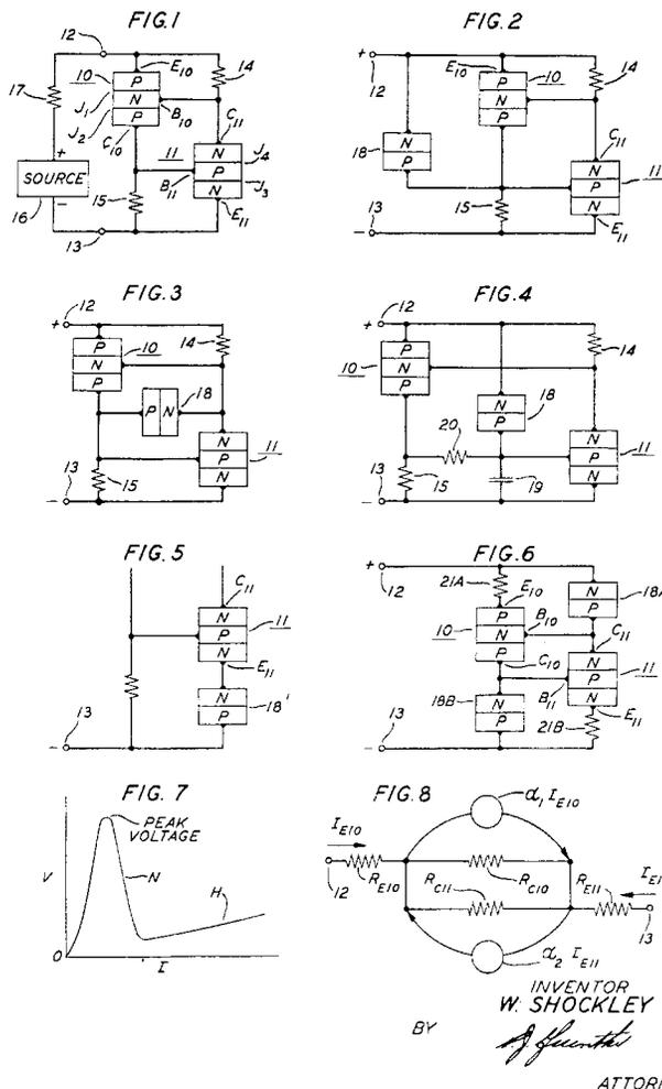
Fig. 14. Shockley's invention of the p-n-p/n-p-n complementary symmetry pair as a bistable transistor switch (U.S. Patent 2 655 609).
