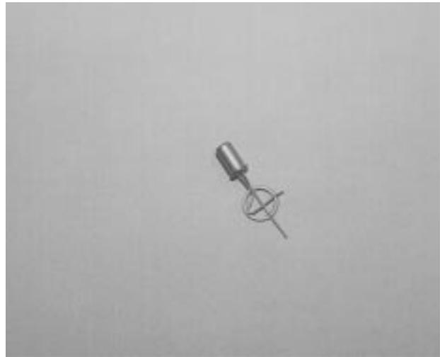
Fig. 20. A picture of the Shockley diode.
