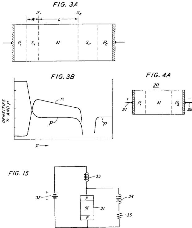
Fig. 10. Shockley's invention of the negative resistance semiconductor device arising out of transit time delay (U.S. Patent 2772360).
