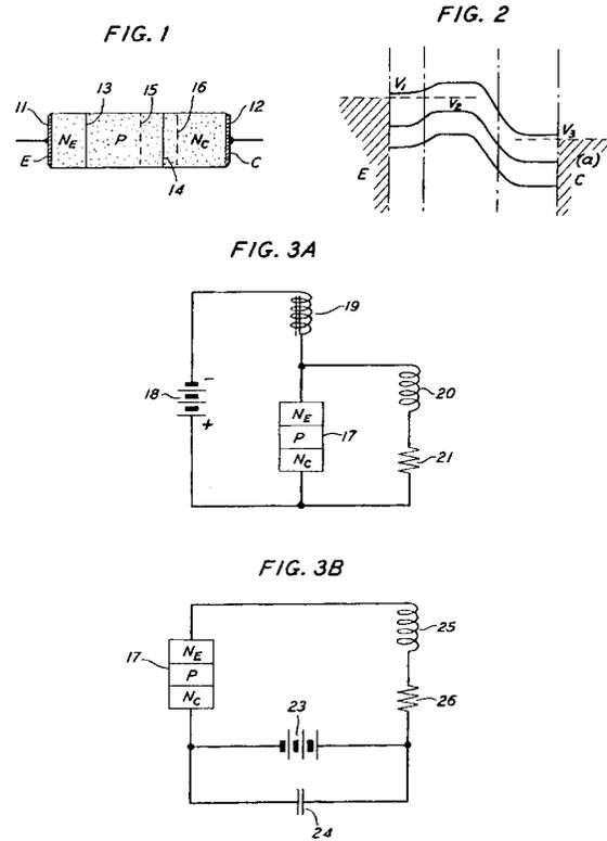
Fig. 11. Shockley's invention of the high-frequency negative resistance semiconductor device arising out of transit time delay (U.S. Patent 2794917).
