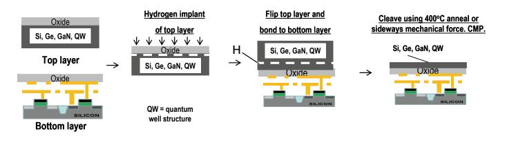
**Create** a layer of Recessed ChAnnel Transistors (RCATs), commonly used in DRAMs, by activating dopants at  $\sim 1000^{\circ}$ C **before** wafer bonding to the CMOS substrate and cleaving, thereby leaving a very thin dopant stack layer from which transistors are completed, utilizing less than 400°C etch and deposition processes.
