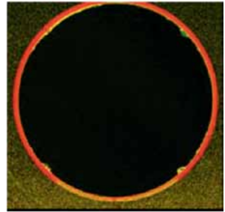
Figure 3a: Acoustic microscope image of the patterned Cu bonding interface (5x5 \mu\text{m} Cu pad size and 10 \mu\text{m} pitch, Cu density 20%) with 2h of annealing at 400°C
