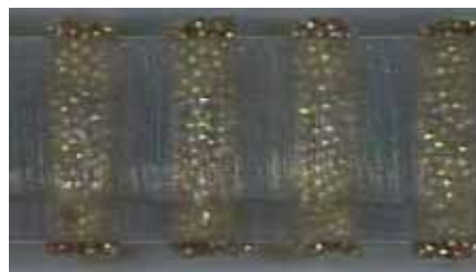
Figure 2: Cross section of SM contacts.
