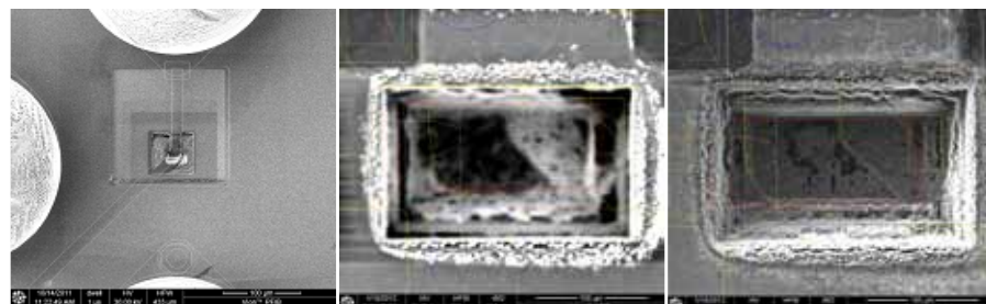
Figure 2: a) (left) CAD data has been overlaid on the FIB image; b) A close up of the access window; and c) The line has been cut and the copper completely removed.
