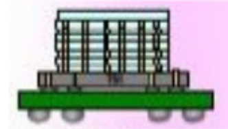
Heterogeneous Multi layer 3D-IC TSV integrated
